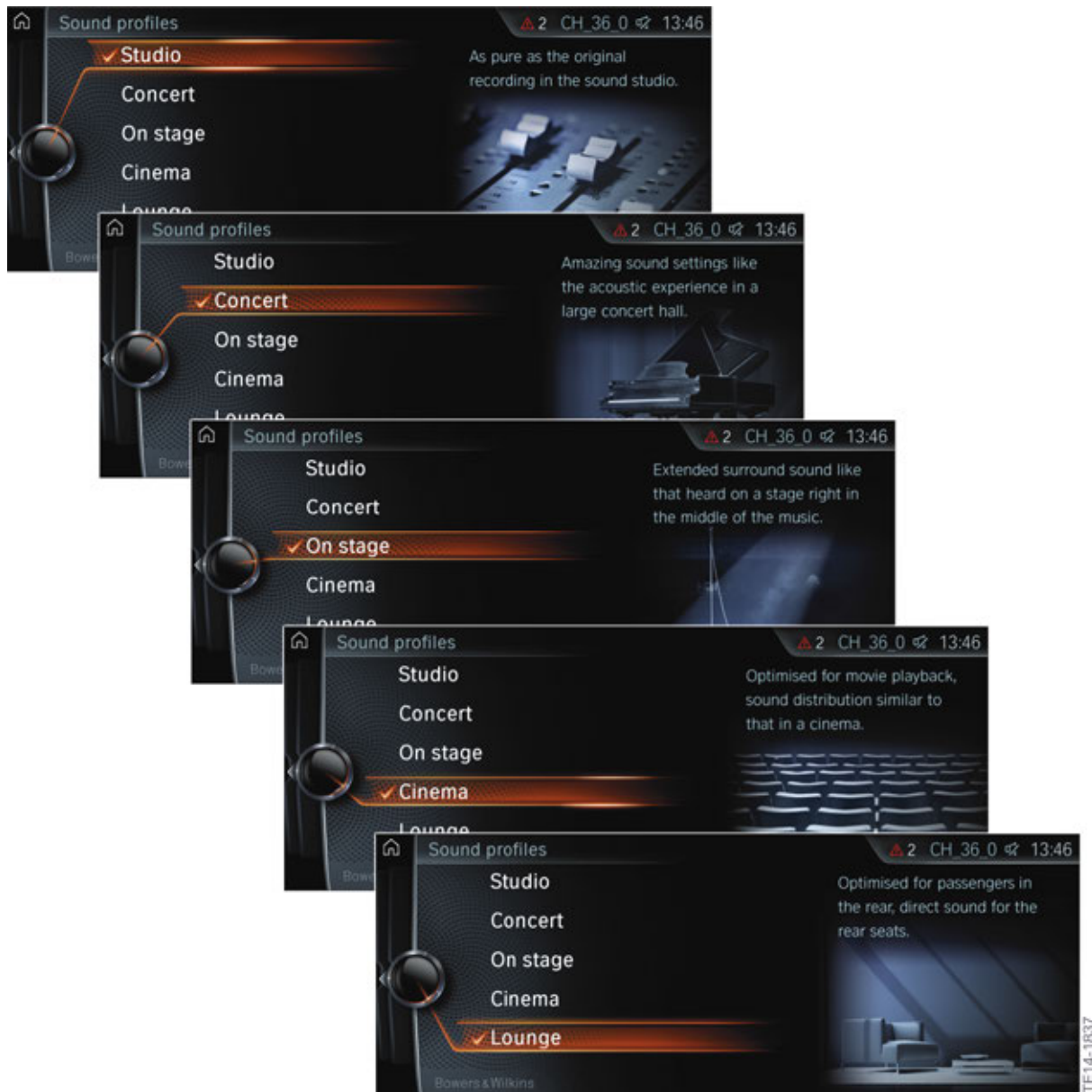
Overview of sound profiles of the Bowers & Wilkins Diamond Surround Sound System
